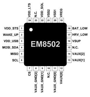
Figure 1 EM8502 QFN24 pins location
