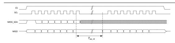
Figure 7-7 SPI transaction for reading the E<sup>2</sup>PROM (CPOL=0)
