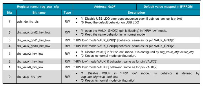
Table 14 "HRV low" mode power switch configuration register (0x0F)
