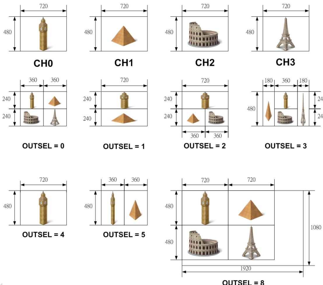
The following table shows the scaling ratios at the horizontal direction and the vertical direction with different 'OUT\_SEL' settings.
