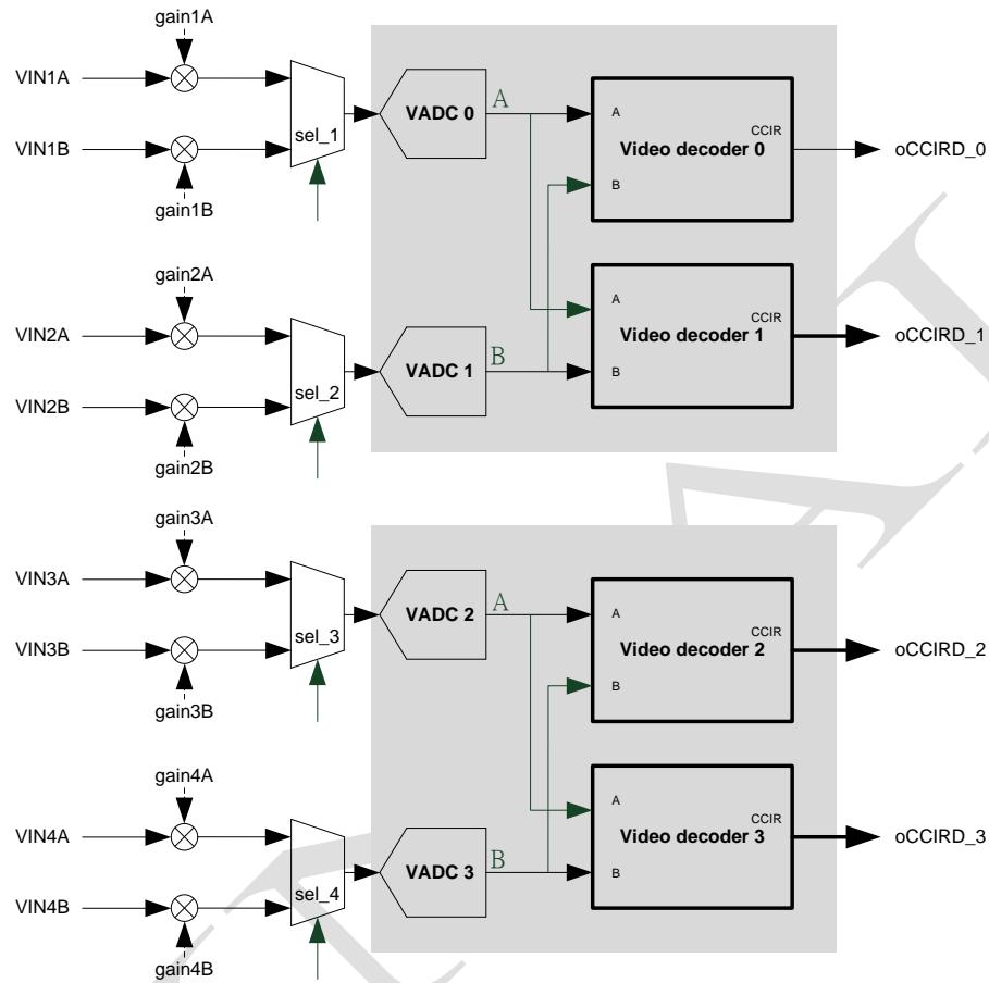
The DM5886 contains four 960H/720H video decoders supporting up to 8 CVBS inputs.
