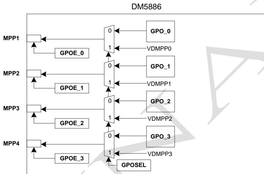
There are four GPO pin (MPP1~MPP4) in DM5886. The GPO function only valid when REG70[4]=0, REG7A[6]=0, **GPOSEL=0 (REG7A[7])** and **GPOE\_X=1 (REG7C[7:4])**. Fig.x shows the GPO function.
