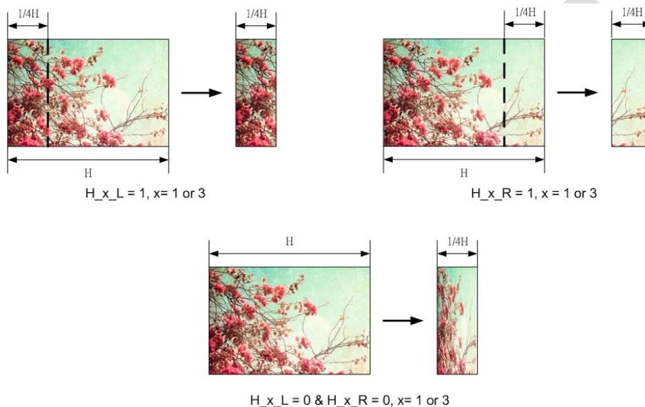
Vertical scaling uses simple line dropping algorithm. No averaging operation is performed. The following figure illustrates the process. Top field is used for output.
