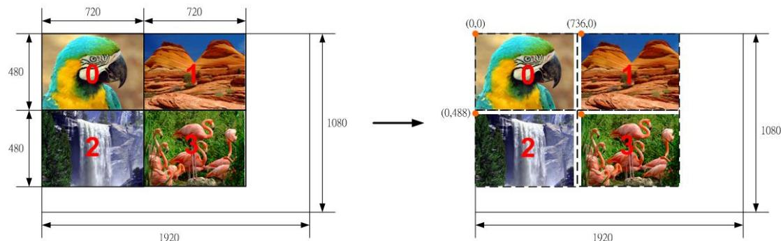
If the input channel is not valid, the corresponding output video will be displayed as blue panel. The following figure shows this condition. The display color of invalid video can also be designed with three registers: 'Blue\_panel\_Y', 'Blue\_panel\_CB', and 'Blue\_panel\_CR' (0xD3 to 0xD5). The default color is blue.
