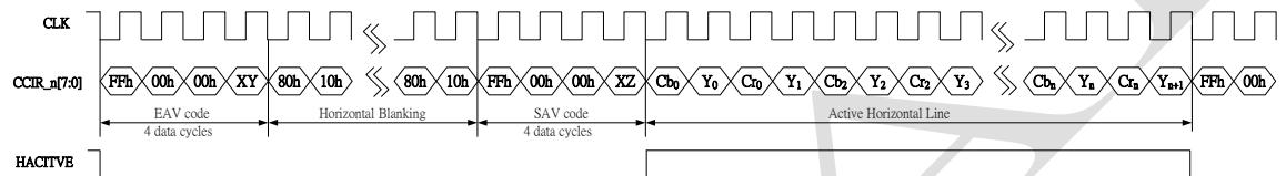
The number of data cycles in active horizontal line will vary according to the output format. For 720H video outputs, the active horizontal line contains 1440 cycles. For 960 H video outputs, the active horizontal line contains 1920 cycles.
