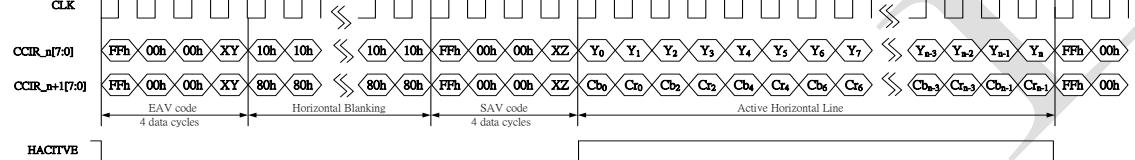
For 1920x1080 HD video outputs, the active horizontal line contains 1920 cycles. The definition of SAV and EAV code sequences is the same as that in 720H and 960H video outputs.
