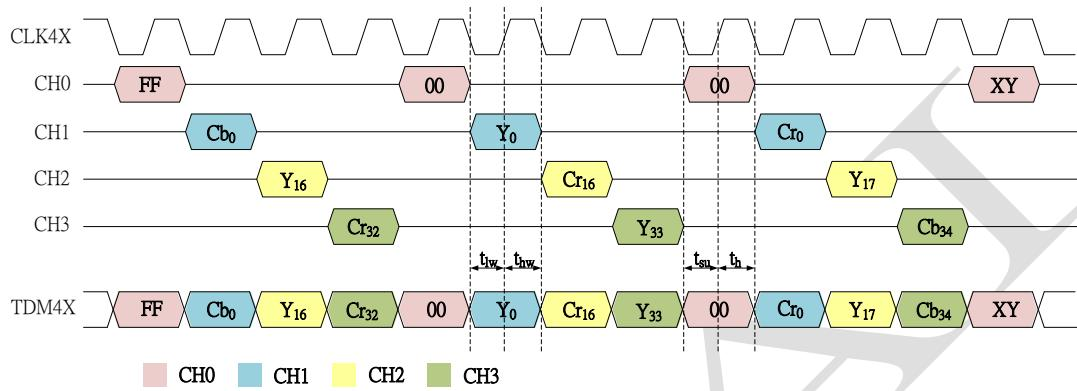
In the Multi-channel Time Division Multiplexing mode, channel IDs are used to indicate the corresponding channels. Channel IDs are defined as the last four bits in SAV/EAV code sequence (i.e. the originally-defined protection bits). The relationship between SAV/EAV code sequence and channel ID is illustrated in the following table.
