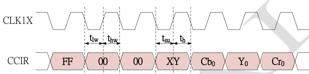
When two-channel multiplexing is selected, two times of the original clock rate is used (54 MHz for 720H video, 72 MHz for 960H video). The timing diagram is illustrated below.
