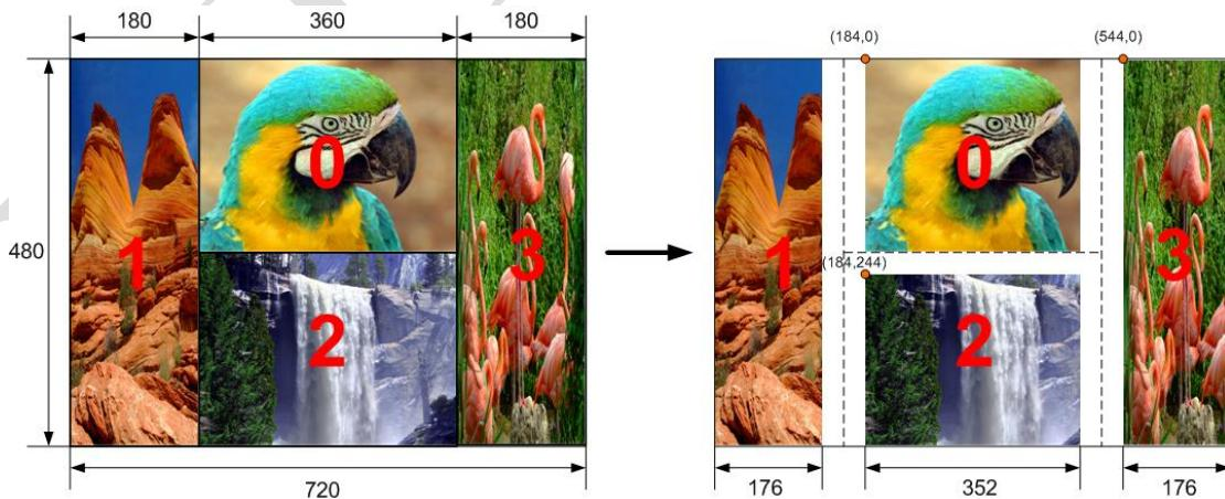
The following figure illustrates another example. The size of input and output video is 720x480 and 'OUT\_SEL' is set to 8 (HD mode). The crop length is set to 704 and it creates horizontal split lines. COR\_X1 and COR\_X3 are set to 736 for center alignment. COR\_Y2 and COR\_Y3 are set to 488 to create a vertical split line with spacing of 8 pixels.
