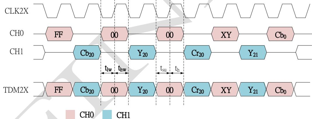
When four-channel multiplexing is selected, four times of the original clock rate is used (108 MHz for 720H video, 144 MHz for 960H video). The timing diagram is illustrated below.
