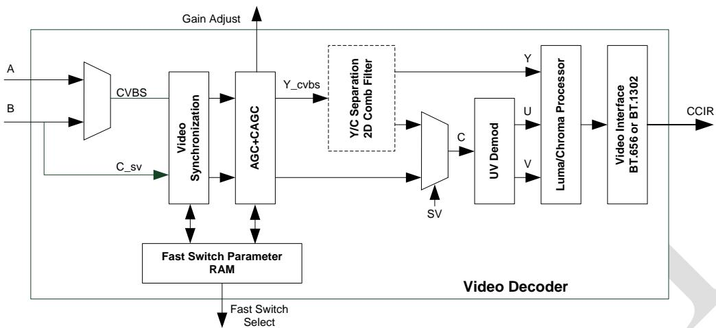
The DM5886 video decoder contains a Video Synchronization block, an AGC block, an YC separation block, a UV Demodulation block, a Luma/Chroma Processor block and a BT 656 output block. A patented Fast Switch is also included.
