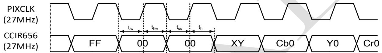
Figure 3-2 . Clocks, CCIR656 Output Data Timing
