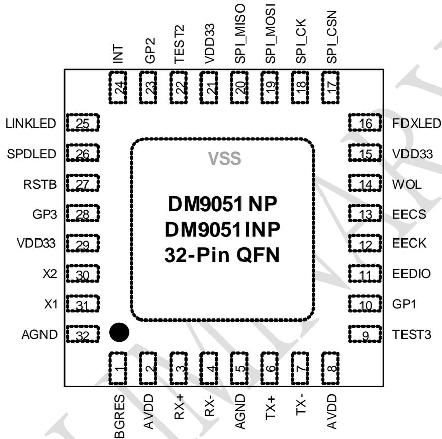
Note: The DM9051(I) IC employs a QFN package, which means the absence of a pin dedicated to ground (GND). In the QFN package, the GND is located at the bottom of the IC directly in the middle. Exposed pad (VSS) on bottom of package must be connected to ground.
