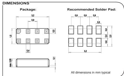
Extremely Accurate RTC Module with embedded Quartz Crystal. Ultra Low Power consumption I<sup>2</sup>C Interface Automotive qualified, according to AEC-Q200 Rev. C
