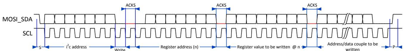
**Figure 7-1: I<sup>2</sup>C write (multiple transactions)**
