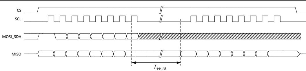
Figure 7-7 SPI transaction for reading the E<sup>2</sup>PROM (CPOL=0)
