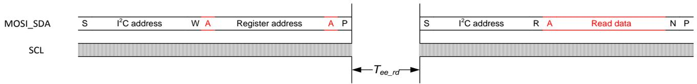
Figure 7-11 I<sup>2</sup>C transaction for reading the E<sup>2</sup>PROM
