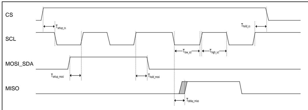
Figure 5-1 4-wire SPI Timing Diagram
