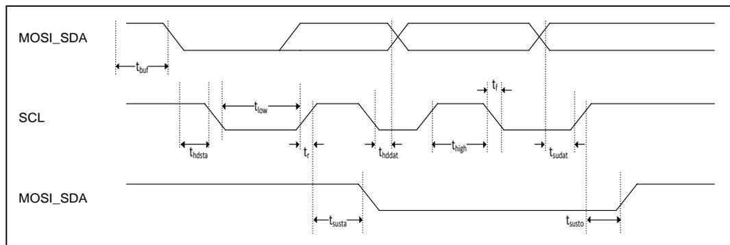
Figure 5-2 I<sup>2</sup>C Timing Diagram
