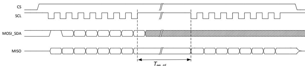
**Figure 7-6 SPI transaction for reading the E<sup>2</sup>PROM (CPOL=1)**
