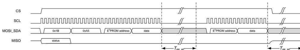
Figure 7-9 SPI multi-byte transaction for writing the E<sup>2</sup>PROM
