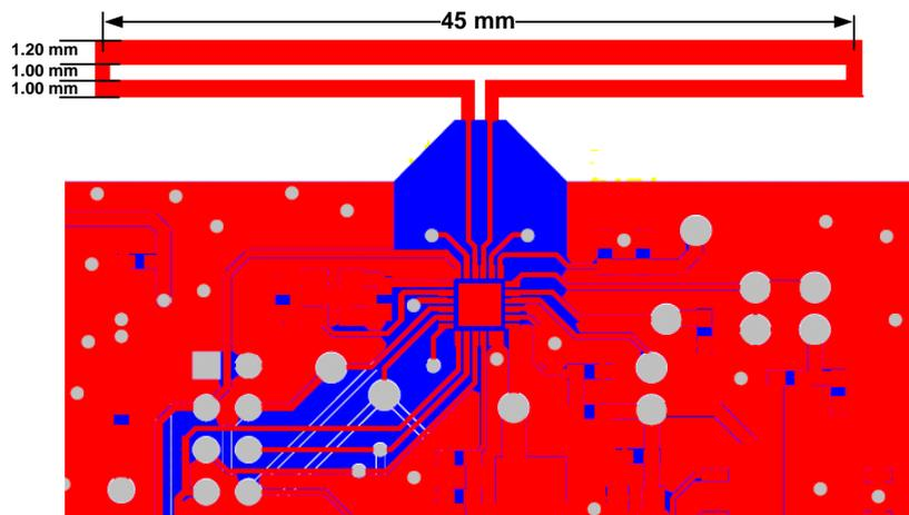
Figure 9.1 Layout example of a folded dipole antenna.
